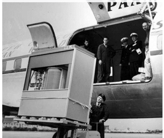
Fig. 11. IBM 350 hard-drive, from 1956, with a capacity of 5 megabytes.
